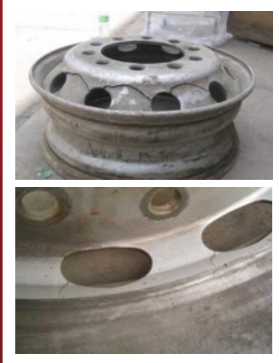
A .Dis broken, wheels overload, poor road condition, sudden braking.
