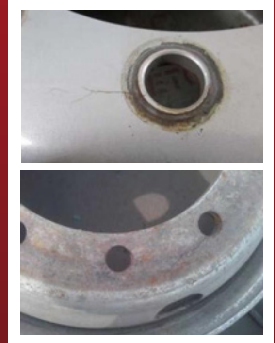
C . Fatigue cracking of bolt hole: the installation is not in place, the bolt torque is not enough or all the bolt torque is not uniform
