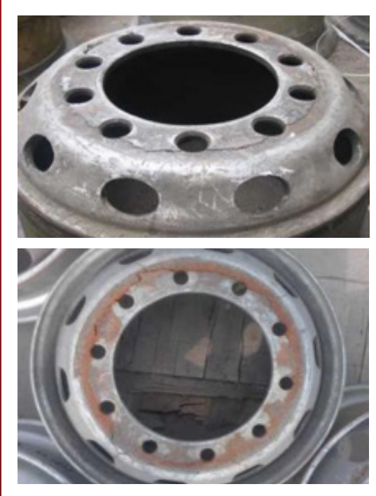
B . The bolt hole crack: Nut looseing, resulting in uneven bolt hole stress, wheel overload, insufficient tire pressure or careless driving,
